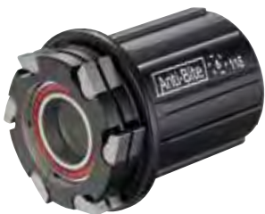
Shimano 10/11s (6 Pawls working together) Aluminum R07T-HHA2 80g ± 5g
